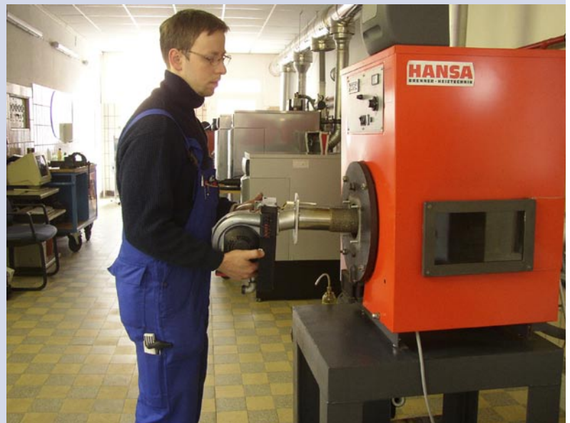
The burner will be put into the boiler in quite a simple way
