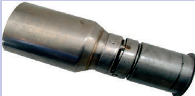
Flame tube and alloy-tube for HB 40 with large recirculation
